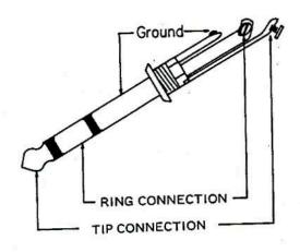
Figure 3. Amplifier Control Plug.
