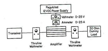
Figure 2. Test Circuit Block Diagram.
